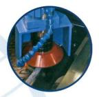
Cup wheel used on press brake dies etc.
