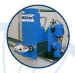
Titable up to ± 30°, manual or automatic downfeed
